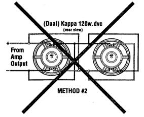
IMPORTANT: When connecting two Kappa 120w.dvc subwoofers together, use Method #1 to create a net 4-ohm impedance, NEVER USE METHOD #2, since most amplifiers cannot fully control driver movement in this configuration.
